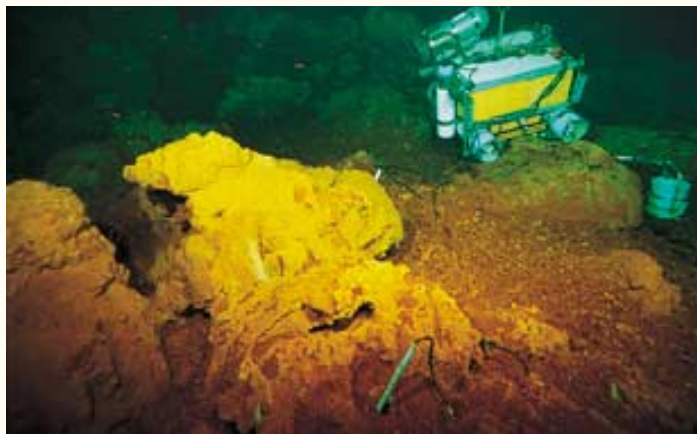
PISCES V SUBMERSIBLE (above, left) is lowered from its support vessel, the Ka'imikai-o-Kanaloa . Ocean-bottom observatory (above) has a time-lapse video camera on top, a seismometer to the right and temperature probes, which are inserted into hot-water vents.
